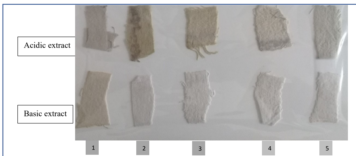
Figure 2: Results of the dyeing control process done on the cotton fabric tinted with the acidic and basic extracts of Brachyotum microdon (flowers). 1 Fabric rinsed with water; 2 Fabric washed and rubbed with water; 3 Fabric washed with a detergent and then rinsed (without rubbing); 4 Fabric washed with a basic detergent and rinsed (with rubbing); 5 Fabric washed with an acidic detergent and rinsed (with rubbing).
