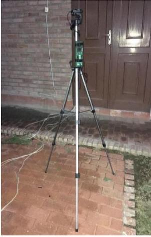
Figure 17: Luxometer on tripod.
