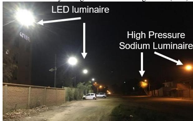
**Figure 16:** The complete deployed pilot system, comparing LED luminaires and High-Pressure Sodium luminaires.
