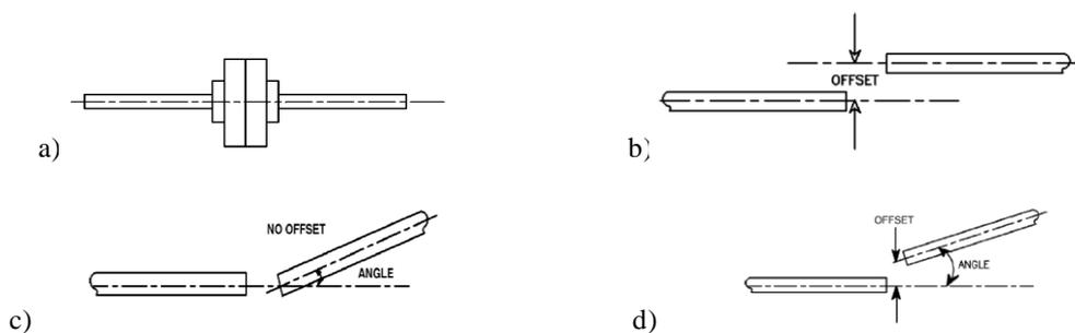
**Figure 1:** Three types of misalignments, a) Alignment shafts, b) Parallel alignment, c) Angular alignment, and d) Combined alignment [16].
