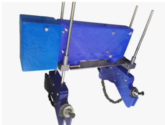
**Figure 2:** Designed and developed measurement system for shaft alignment.
