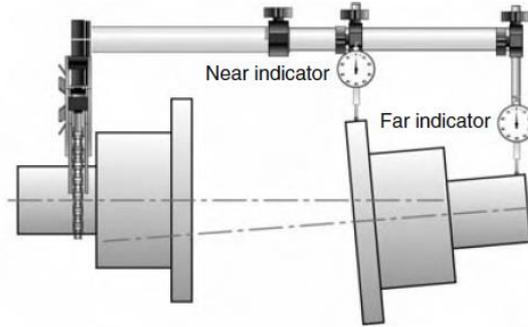
**Figure 7:** Arrangement for radial alignment method [18].
