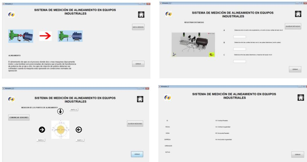
Figure 11: Monitoring system by using the graphical interface user (GUI) in Matlab®.
