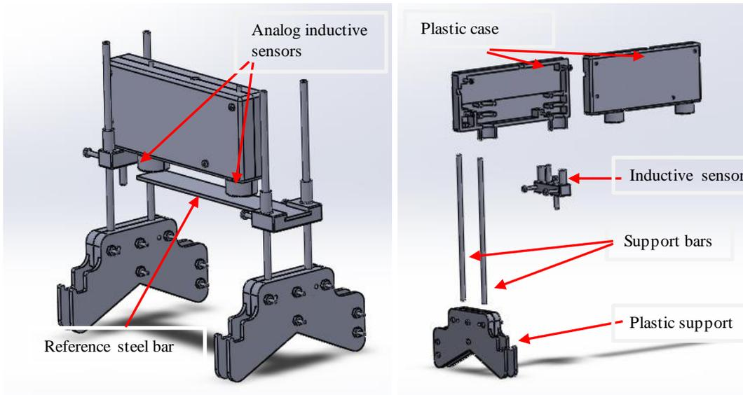
Figure 5: The 3D design of the mechanic components.
