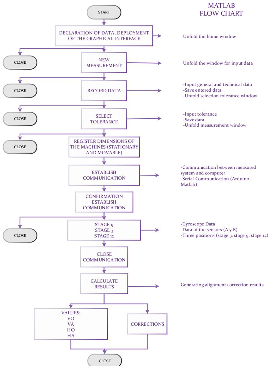
Figure 6: The software programming framework of the shaft alignment analysis procedure.
