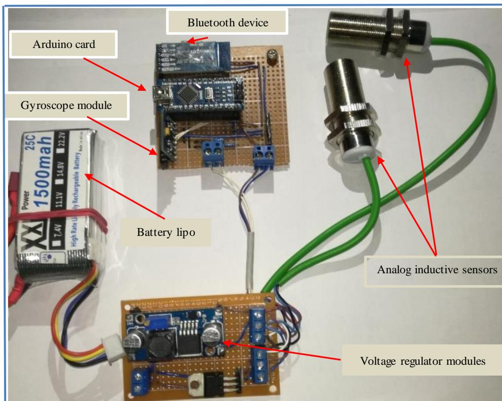
**Figure 4:** Developed measurement system.
