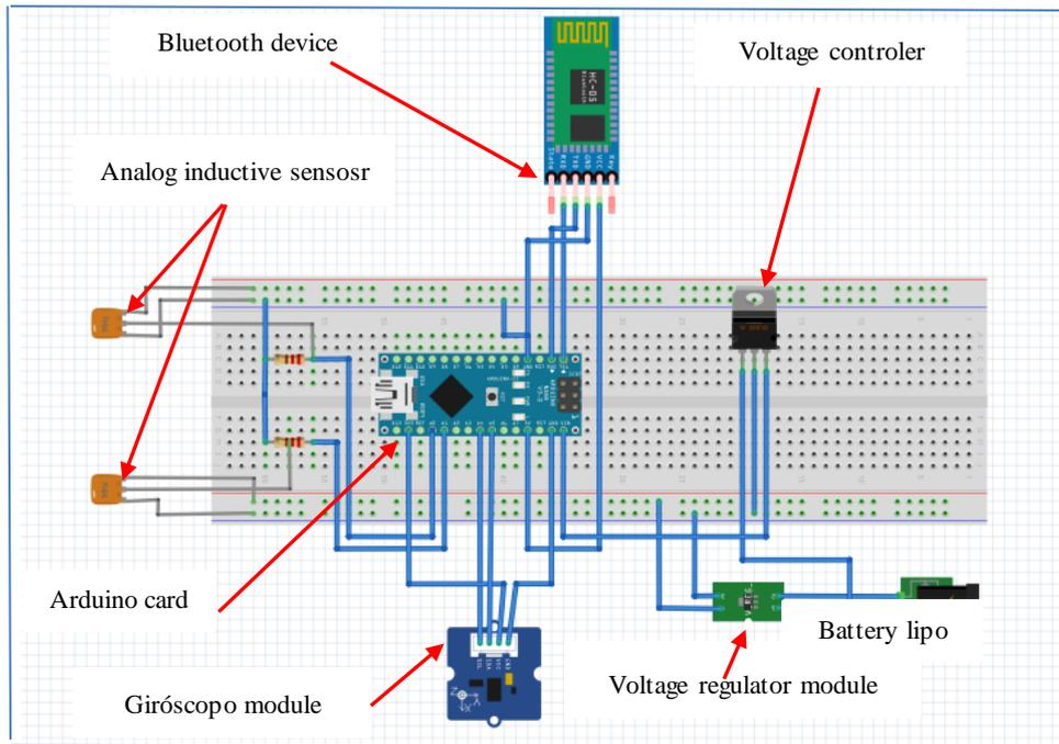
**Figure 3:** Schematic diagram of the electronic circuit.
