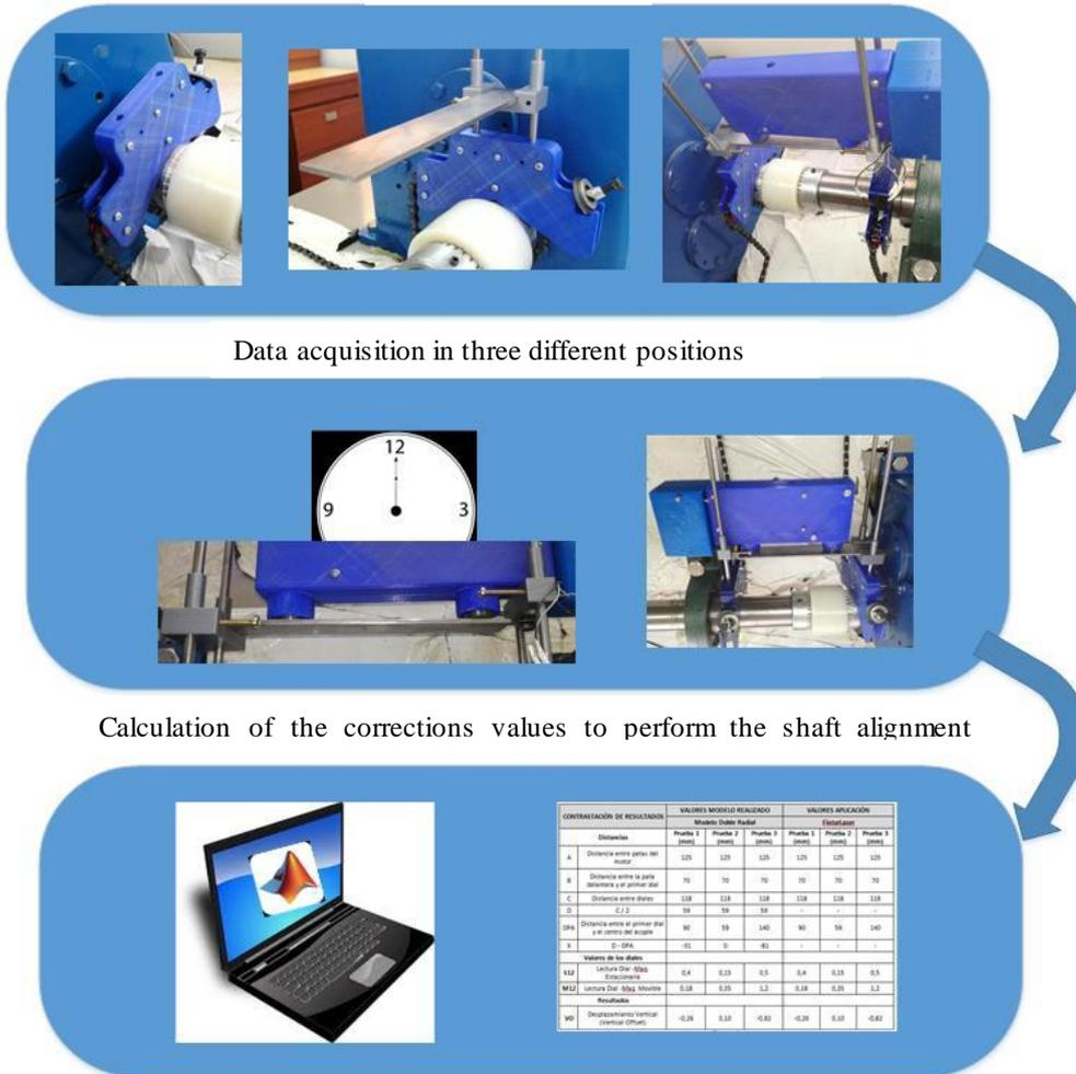
Figure 10: Overall structure for determination of the shaft misalignment system.
