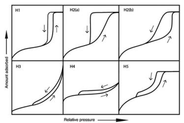
Figure 2. IUPAC Classification of adsorption-desorption hysteresis loops [12, 17].
