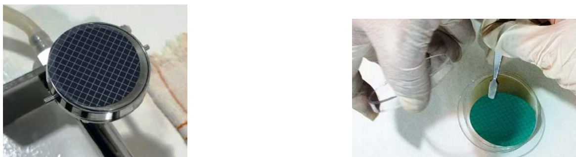
Photo 1. Sample filtration. Membrane in the culture medium Own source: Juan Carlos Surco Almendras
