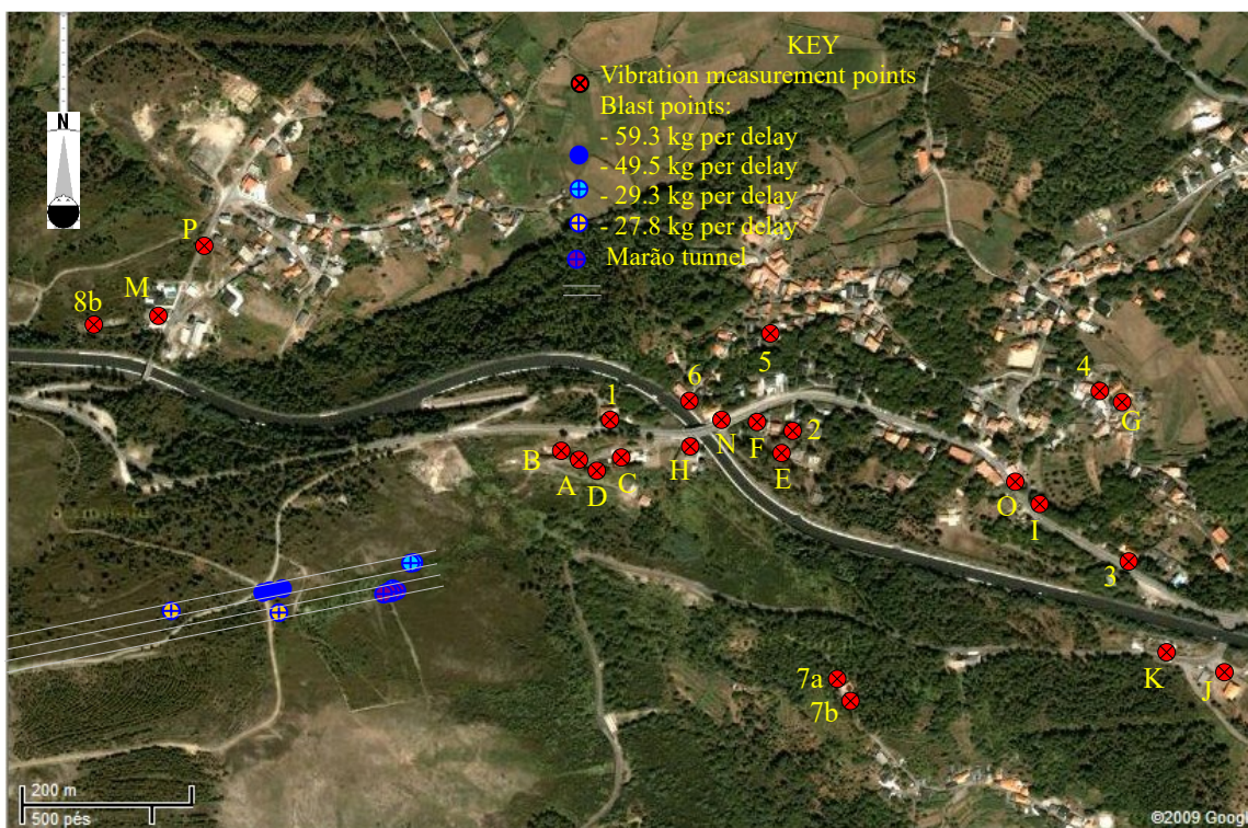
Fig. 6 Vibration measurement points and blasting points
