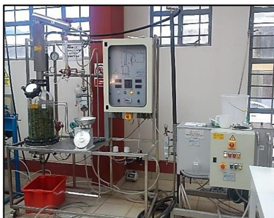
Figure 1 Steam injection entrained distillation process
